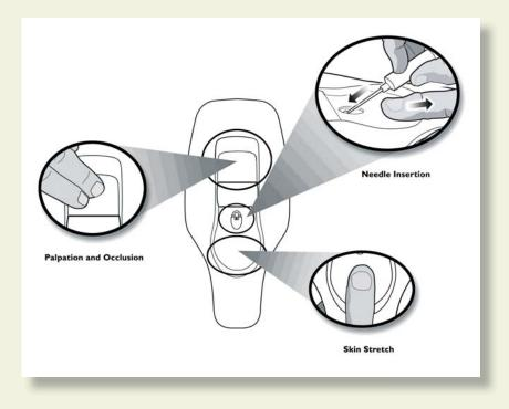
The following schematic depicts the various parts and functions of the haptic device, shown from above. The device should always be placed on a flat, level surface.
