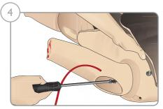
4. Secure the Adapter with one hand from inside the torso. Screw the Adapter Screw using the Phillips screwdriver:
