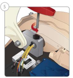
5. Unscrew the left Arm screw with the allen key and disconnect all Arm cables.
