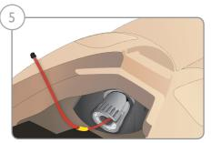
5. Insert the blood tube into the side slot of the connector. Screw the connector in place with one hand.
