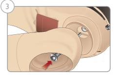
3. Thread the Adapter Screw through the Amputation Arm and align the screw with the hole in the Arm Adapter:
