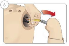
6. Remove the arm with cables from the arm socket.
