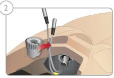
2. Unscrew hip joint connector. Remove the leg cables/tubes from the connector.
