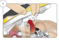
Lift the hinged chest plate to access the arm bolt.
