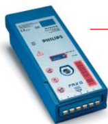
M3848A FR2+ Rechargeable 12VDC 1.6Ah Li Ion Battery. (This battery is fully charged in 3 hours, to provide 100 shocks (typical) or 5 hours ECG monitoring (typical). This product is compatible with FR2 defibrillators sold after 12/1/01 only. To use with an earlier FR2, your FR2 must be upgraded. Not all older FR2s are eligible.
