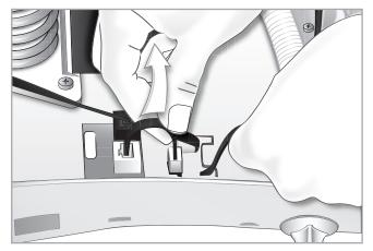
4 Remove the 4 retaining screws and discard the old sensor unit.
