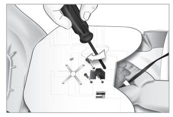
7 Route and reconnect sensor cables back to the lung plate and side connection unit board, as shown on step 3. Reinstall lung plate as shown in step 2 and re-attach manikin chest skin.
