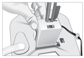
**6** Install 4 retaining screws to the new sensor unit as shown below.
