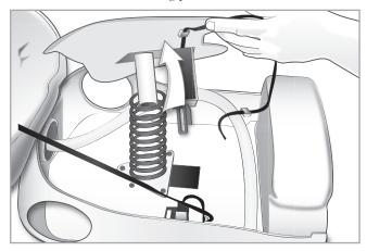
**3** Remove the cable with strain relief from the lung plate and the side connection unit board as shown below.
