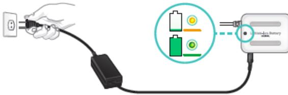
During charging, the LED indicator on the battery will show a steady yellow. When the battery is fully charged, the LED indicator shows steady green.
