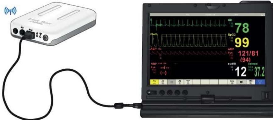
A wired connection to the Patient Monitor is the recommended connection method. A wired connection ensures continuous transfer of data and no interruption in waveform drawing on the monitor.
