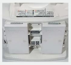
Two rechargeable, lithium ion batteries, when new and fully charged, provide up to 10 hours of monitoring, more than any other monitor/defibrillator. Depleted batteries can be charged to full capacity in just 3 hours. No conditioning is required. Capacity gauges on the monitor's screen and on each battery pack show the remaining charge.
